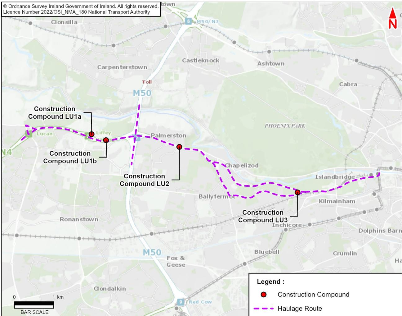
**Diagram 6.6: Proposed Construction Routes and Potential Construction Compounds**
